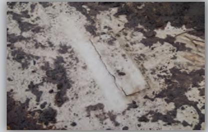
**Location of the leak:** Roof of gasoline storage tank. Repair replaced temporary patch.
